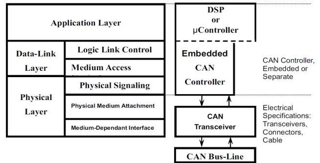
Figure 2 The Layered ISO 11898 Standard Architecture
