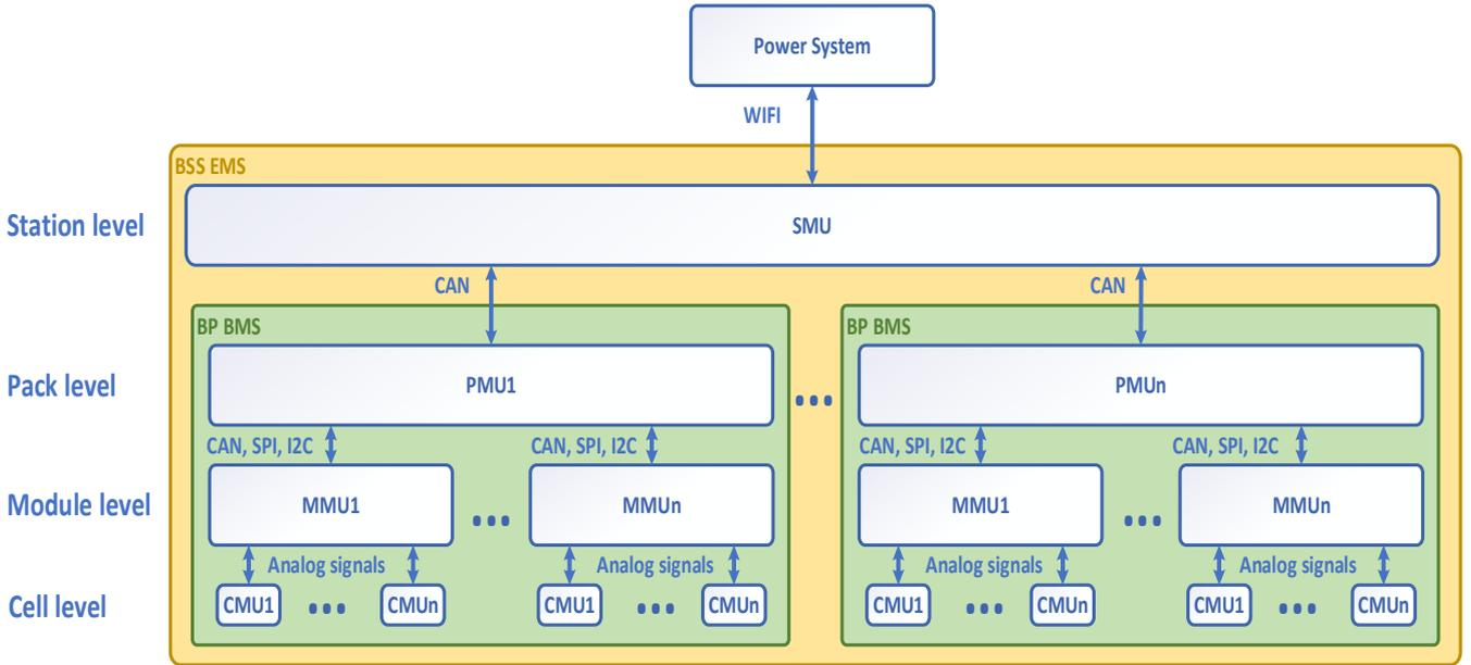
Figure 1 Communication between different nodes within battery packs and swapping station
